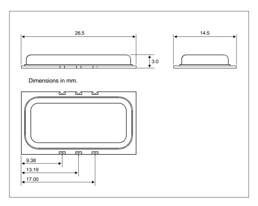
DOCUMENTATION ERROR: The above picture show the ESD protective can with round corners. The TRNG9880 have 90-segree square corners. This will be corrected in next documentation update. The module size and landing pattern is correct
